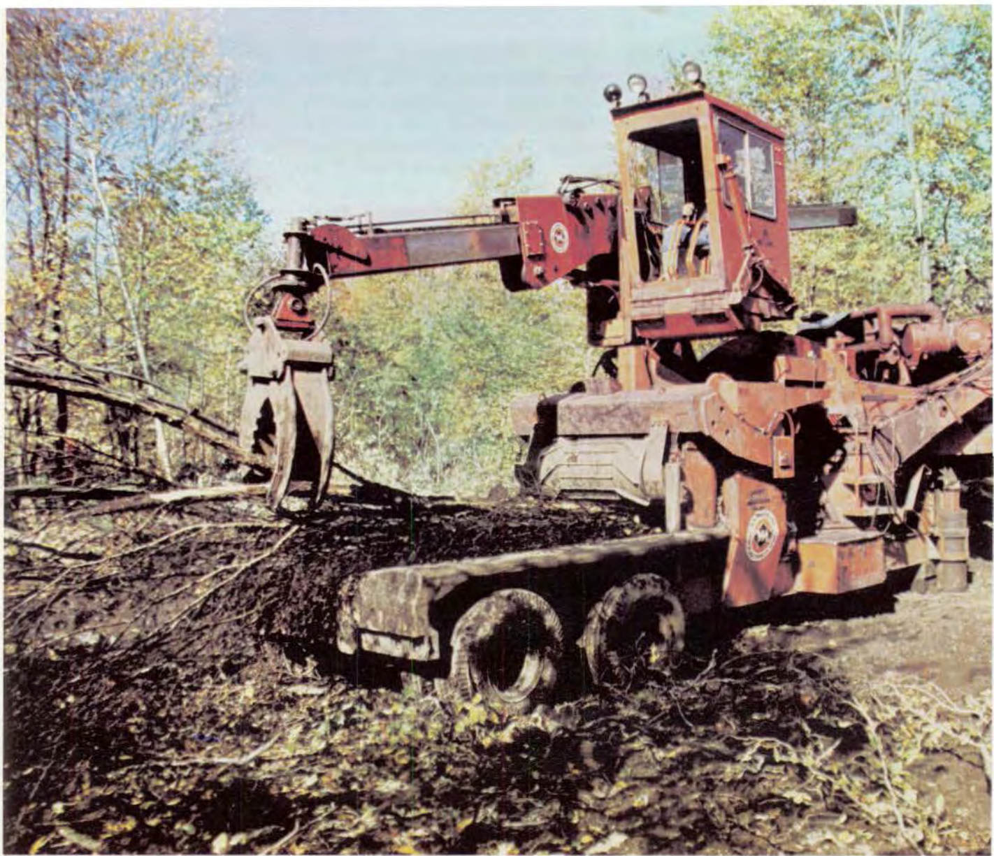
This Morbark wood chipper can effortlessly chew up a 22-inch diameter tree.
