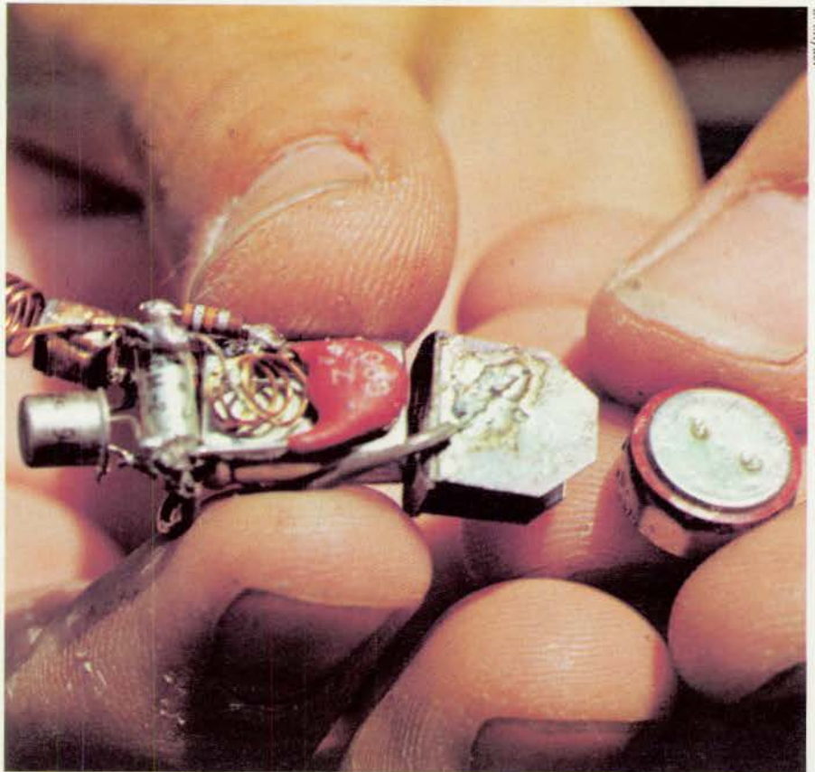
(Above and below) A portable magnetic field is induced by current in wires on the pigeon's head and neck which overrides the natural magnetic fields.
