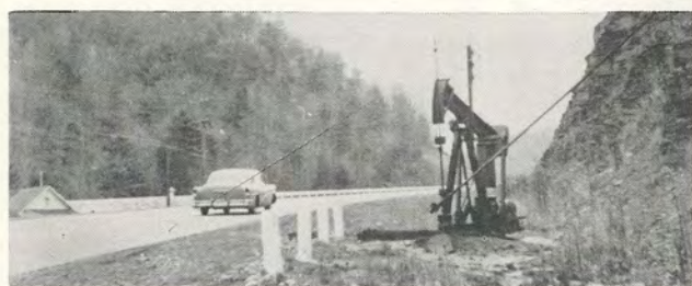
Electrically driven well near Allentown, N. Y.
