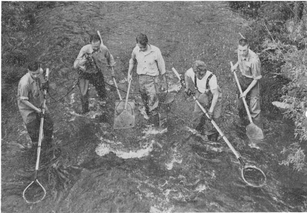
Figure 2. Electrofishing with direct current, the negative terminal floating (center, beneath dip nets) and the positive terminal consisting of two charged dip net rims.
