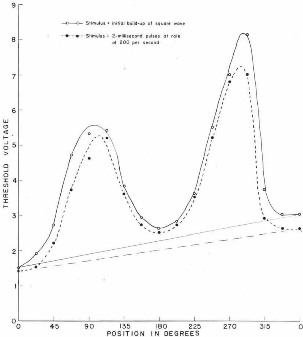
Figure 2. Variations in threshold voltage required for different positions of test fish with respect to axis of electrodes for two types of direct current stimulus. Zero degrees represents fish with head pointed toward positive pole.
