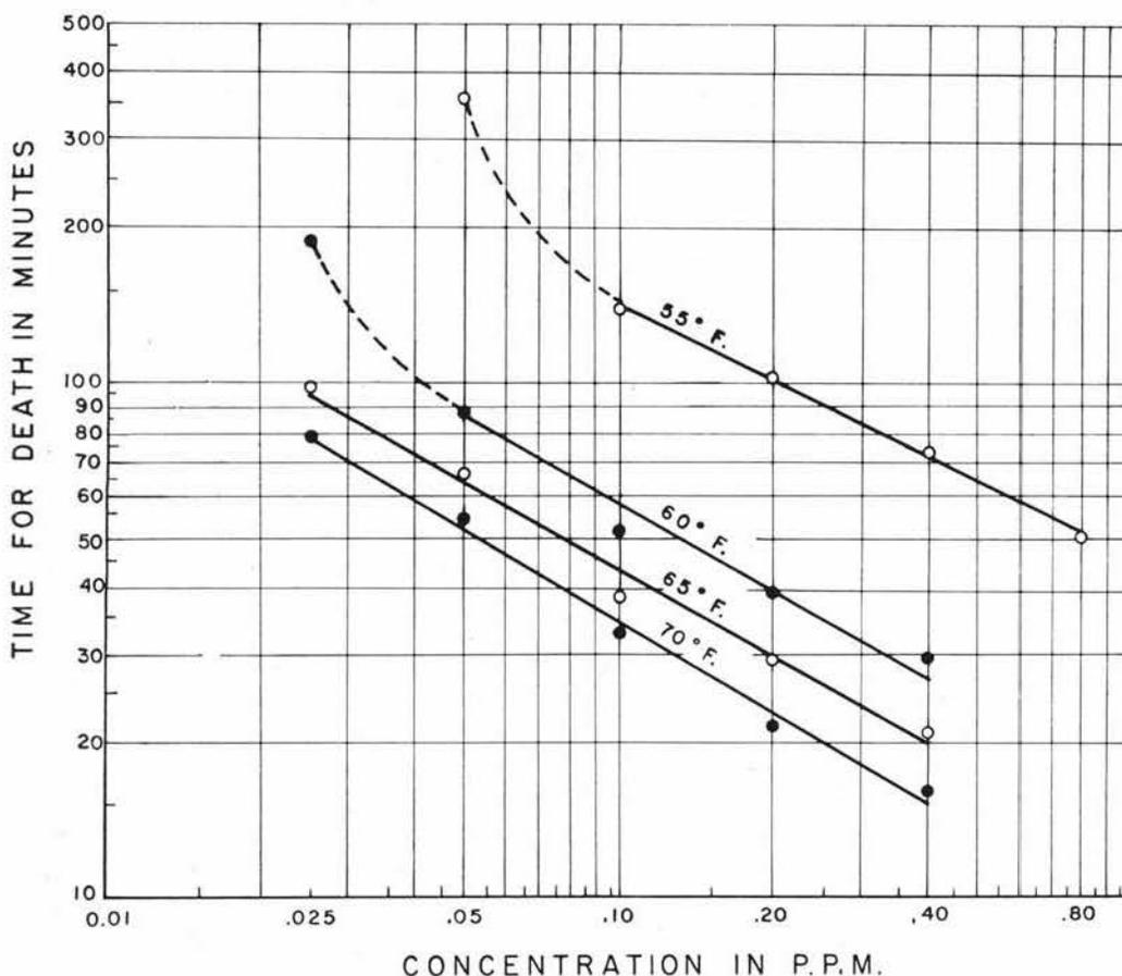
Figure 4. Comparison of the toxicity of rotenone to brown trout fingerlings at different temperatures. The solid lines represent the regression of the plotted means and the broken lines represent extensions to points obviously departing from the straight line. Solid circles and open circles are used merely to differentiate between the sets of data.
