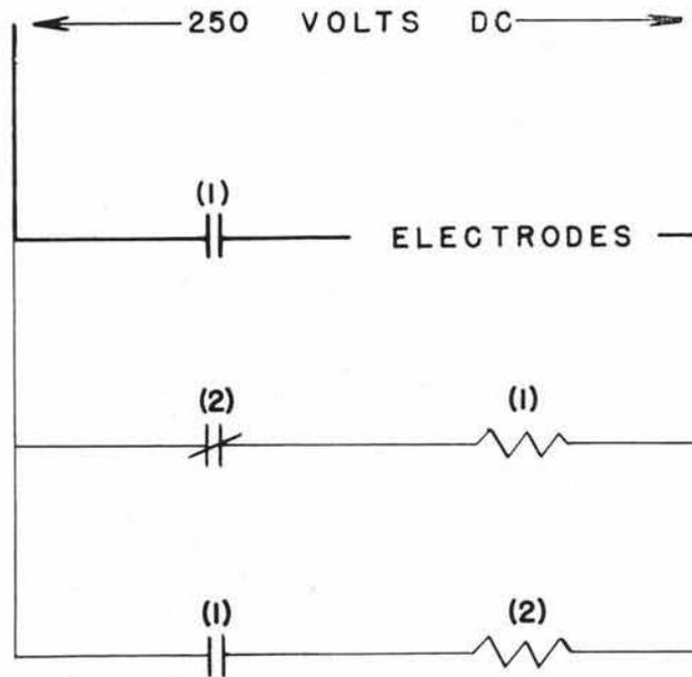
Figure 7. Schematic diagram of circuit used to produce 0.8 second on and 0.2 second off sequence by means of two General Electric contactors (CR 2820-1054) set for 0.8 second drop out (1) and 0.2 second drop out (2).
