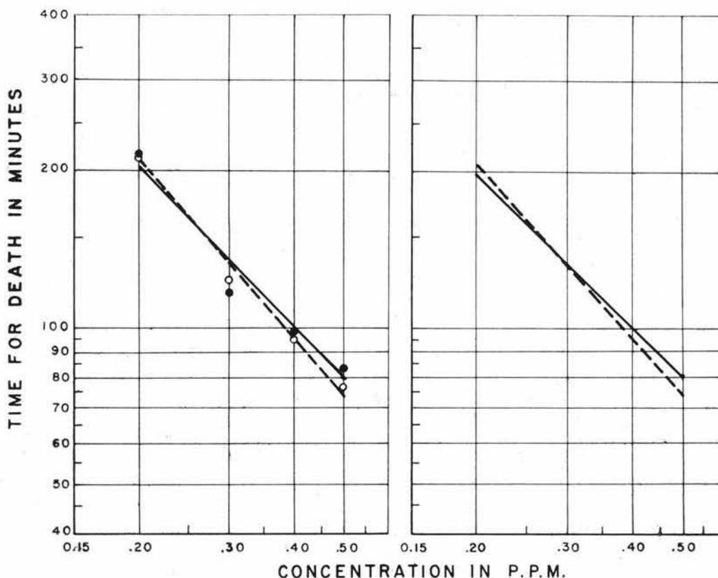
Figure 1. Toxicity curves for creek chubs in acid water (solid line) and alkaline water (broken line): plotted means and their regression (left); regression corrected to a mean length of 53.16 millimeters (right).
