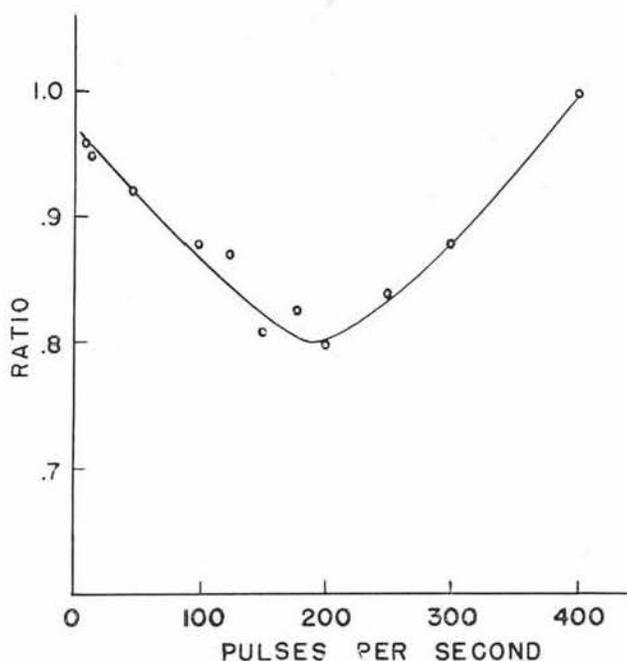
Figure 1. Variation in the ratio between the threshold voltages for pulsating and for steady direct current (in terms of the latter) at different rates of pulsation.
