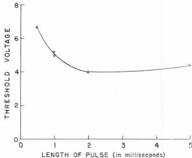
Figure 3. Relation of length of pulse to threshold voltage for direct current having a pulsation rate of 180 per second.
