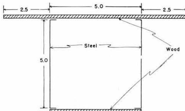
Figure 2. Design of net mouth showing location of metal sides used as electrodes. Dimensions in feet.
