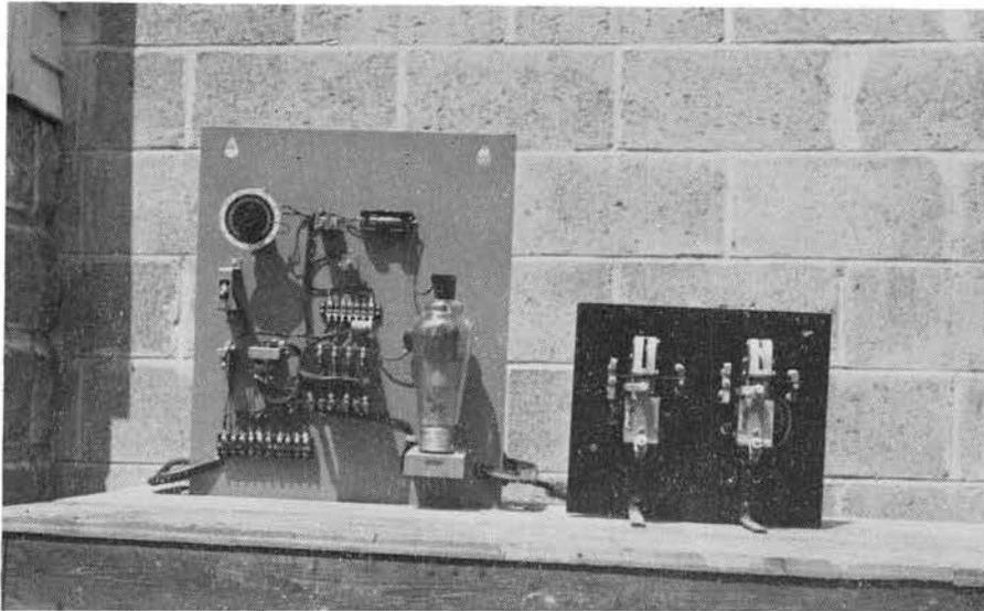
Figure 6. Equipment for producing pulsating current: (left) welding panel used to produce a rapid cycle; (right) contactor panel used to produce a slow cycle.
