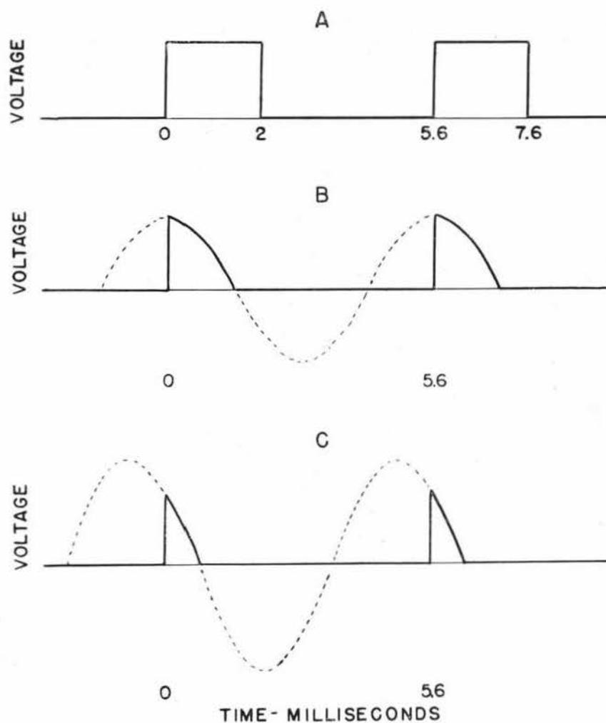
Figure 5. Types of wave or pulse studied in connection with rapid and combined cycles: A, square wave; B, quarter-cycle sine wave; C, eighth-cycle sine wave.
