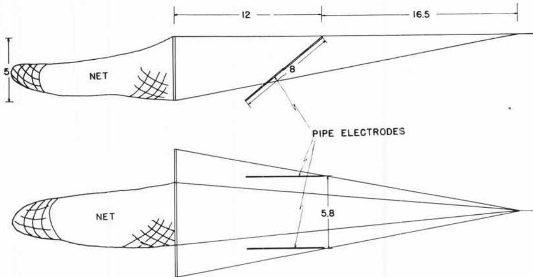
Figure 1. Design of trawl: side view (above); top view (below). Dimensions in feet.
