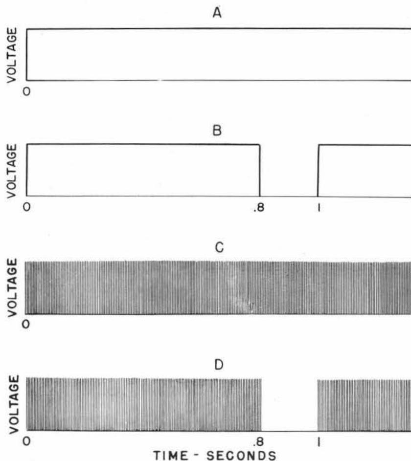
Figure 4. Types of direct current cycle studied: A, steady current (no cycle); B, slow cycle using continuous square wave at rate of 0.8 second on and 0.2 second off; C, rapid cycle using continuous pulsation of 180 per second; D, combined cycle using pulsation of 180 per second at a rate of 0.8 second on and 0.2 second off.
