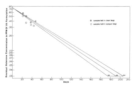
Figure 4. Detoxification of 0.75 ppm of rotenone formulation at 11.3 meters (37 feet). Lines indicate detoxification rates obtained from equation (4) using temperatures of 8° C., 8.3° C. and 9° C. The range of temperatures
