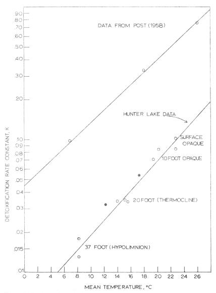
Figure 5. Rotenone detoxification rate and temperature. Upper line (from equation 11) is typical of lighted surface conditions as studied by Post (1958). Lower line (from equation 1) represents deep and opaque samples from Hunter Lake. Dark circles represent data from Marking and Bills (1976).
