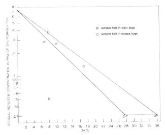
Figure 1. Detoxification of 0.75 ppm of rotenone formulation at the surface of Hunter Lake. Lines indicate detoxification rates obtained from equation (4) using maximum and minimum surface temperatures of 24° C. and 22° C., respectively. Detoxification time shown for clear bags is maximal for this treatment.
