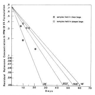
Figure 2. Detoxification of 0.75 ppm of rotenone formulation at 3 meters (10 feet). Lines indicate detoxification rates obtained from equation (4) using temperatures of 18° C., 18.8° C., 20.2° C. and 24° C. The range of temperatures observed was 18° C. to 24° C., and the range of mean temperatures for individual tests was 18.8° C. to 20.2° C.
