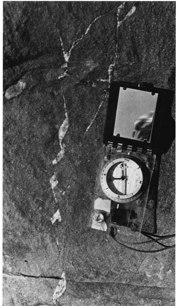
Figure 47. Micro-faults (gash fractures) filled with calcite. The pattern probably reflects the larger one in the westerly adjacent Lake George West Fault. Ticonderoga Dolostone; on north side of access road between Interchange 22 and N.Y. 9L, north of Lake George Village.
