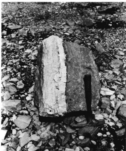
Figure 57. Close-up of loose block in above quarry showing two facies of formation – a darker gray quartzitic facies and a light gray to tan-white friable sandstone.
