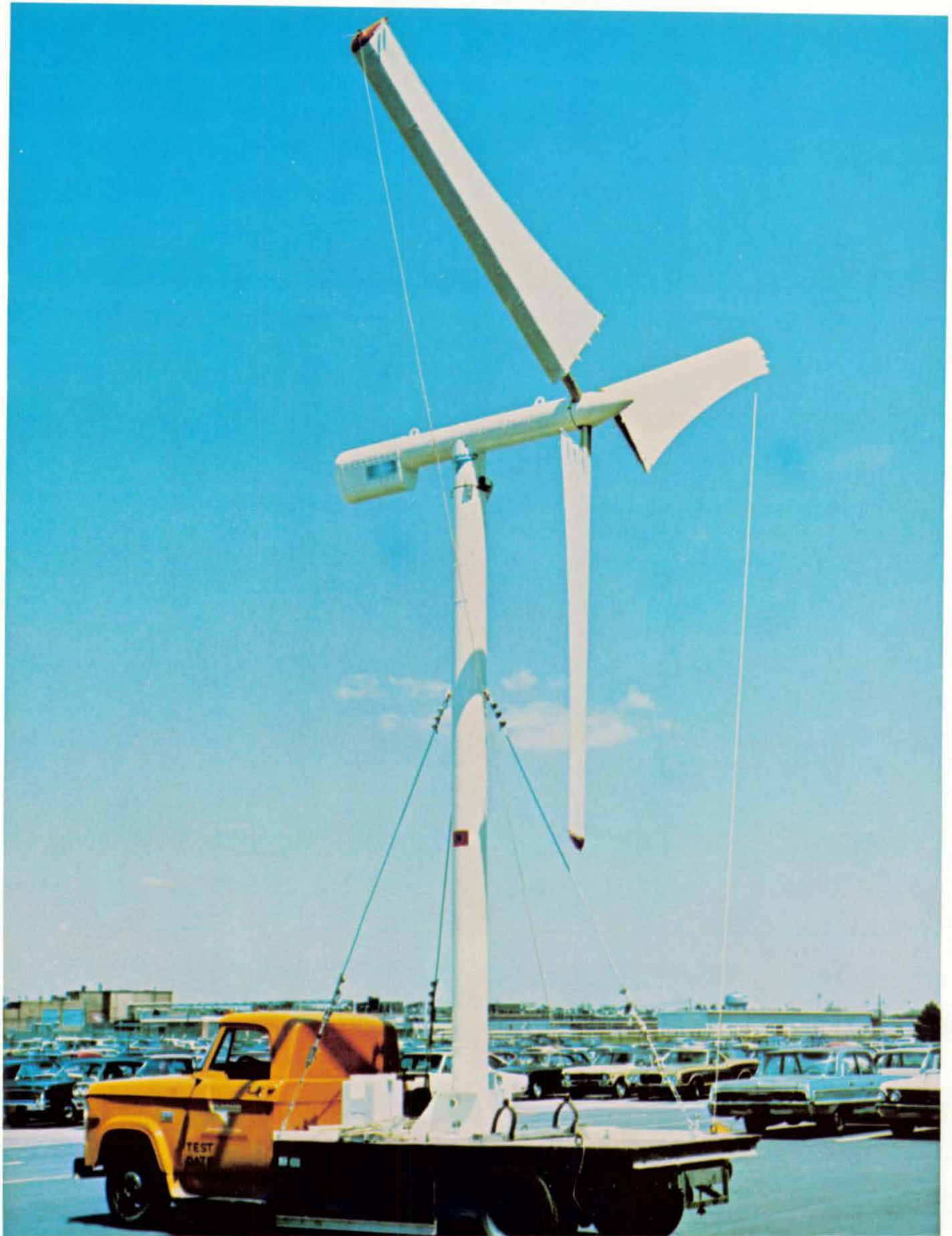
Six-kilowatt home-sized Sailwing wind generator, soon to go into production by Grumman Aerospace Corporation. It is here mounted on a truck for testing at Grumman's Calverton, Long Island, facility. See EQ News Supplement.
